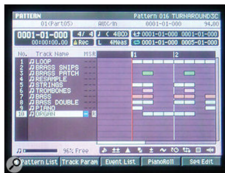
The main Pattern screen has much in common graphically with that of a software sequencer, displaying not only MIDI tracks and their contents, but also a great deal of status information about the Pattern as a whole.
